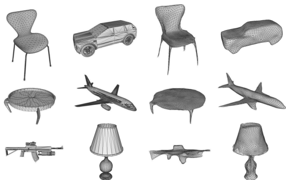
Figure 3. Qualitative results of meshes from Pixel2Mesh. Left two columns are ground truth while right two columns are outputs
